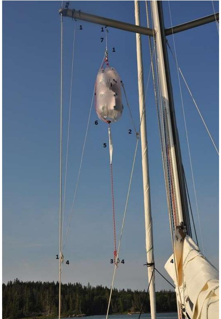
In practice, I don't adjust the reflector port/starboard unless the weather conditions are poor. Even then, it's rare that I do as the reflector does a fine job of staying level on its own unless I am heeling more than 8 degrees.
