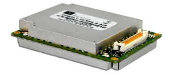
This is the world's smallest Class B (smaller than a standard credit card), yet also the best performing and feature rich fully integrated AIS Class B engine. The device supports both the CSTDMA and pending SOTDMA IMO Class B standards and includes multiple integrated features such as SD and SIM card support and device multiplexing to name only a few.
